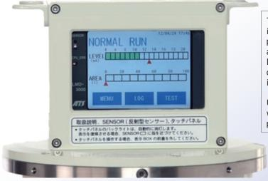
The LMD-3000 detects a film of oil on water surfaces in drainage ditches, pits, oil water separating tanks, purification plant water inlets, etc., and generates an
