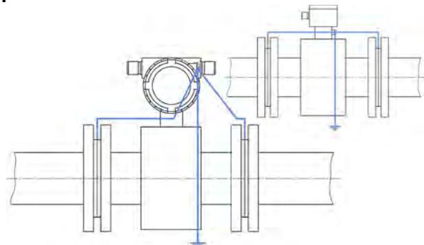
Protection washers or protection rings can also be used as earthing component; or special earthing electrodes, incorporated in the sensor, may be installed.
