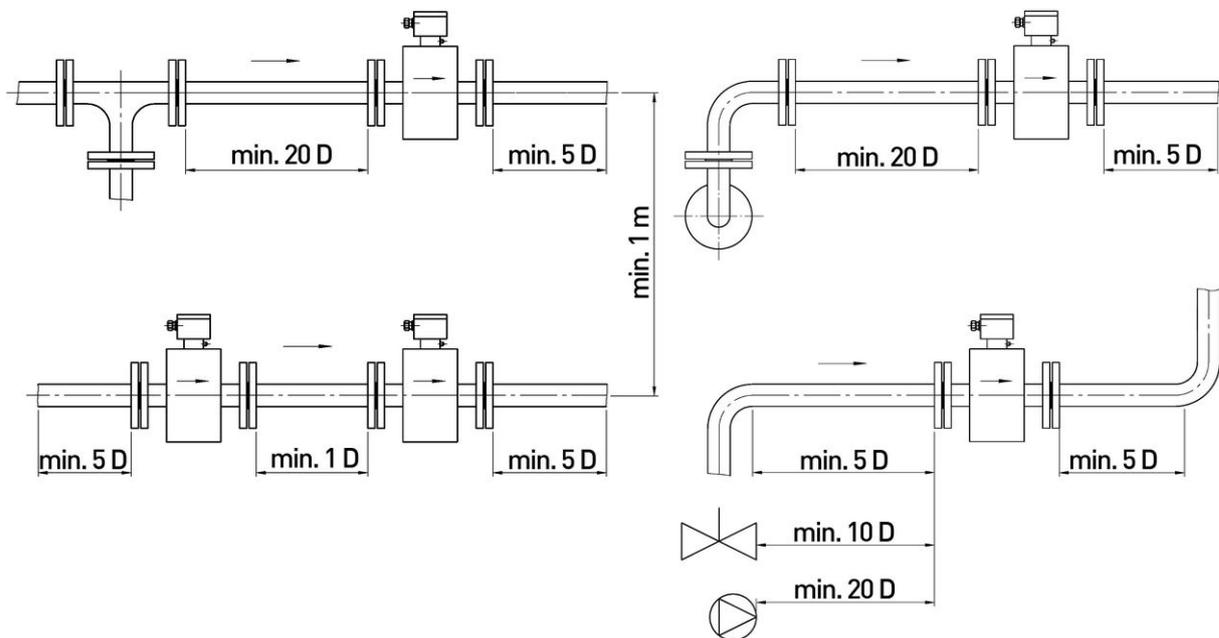
If several sensors are installed in series, the distance between each sensor must be equal to the length of one sensor. If two or more sensors are to be installed in parallel, the distance between sensors must be at least 1 m.
