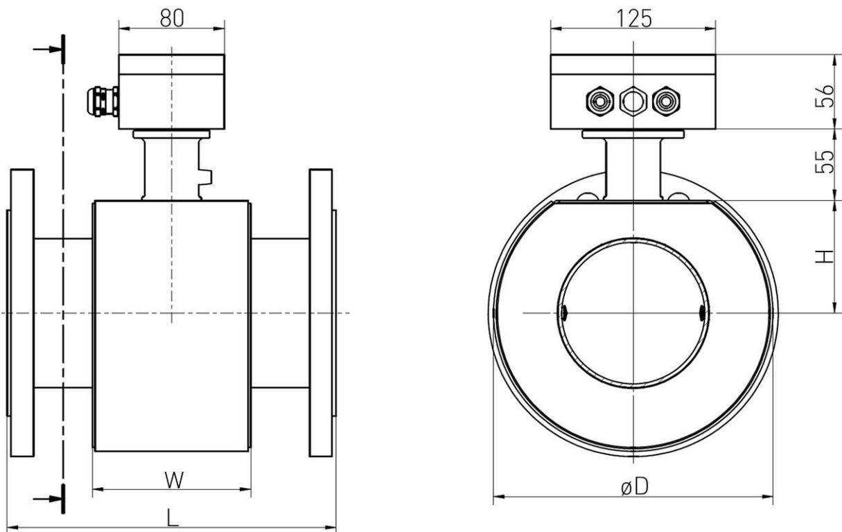
The dimensions L, W, D and H correspond to the values of the table on the compact device (→ § 11.3.1).
