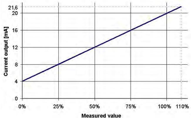
The range from 4 to 20,5 mA is according to the NAMUR-recommendation and uses the measuring range up 104%.
