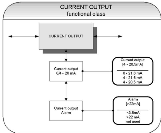
The current output is generally assigned to volume flow.
