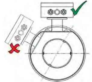
**Installation in unfilled pipeline:**
