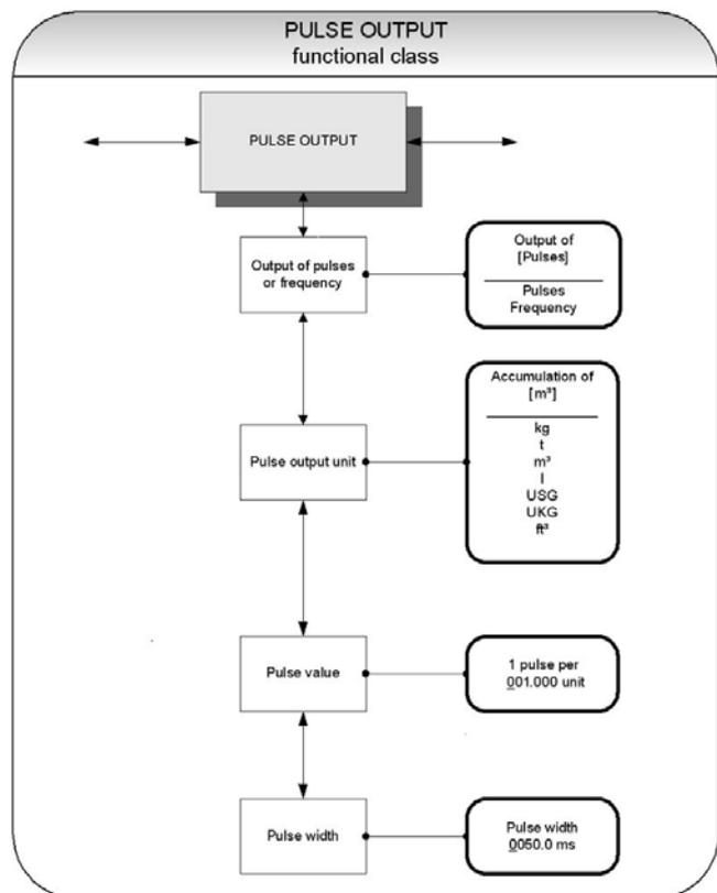
The function *Pulse or frequency output* is used to define the mode for the digital output – either pulses per flow unit or a frequency 0 to 1 kHz corresponding to the measuring range.
